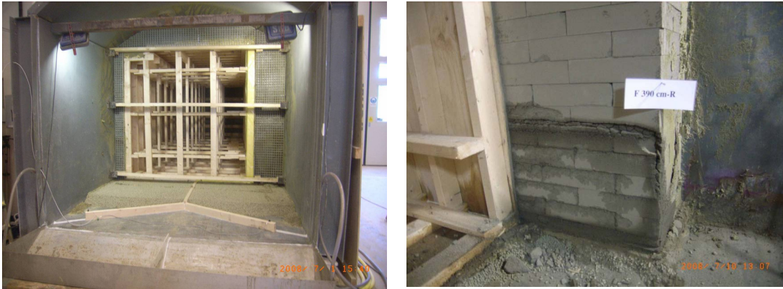
Test set-up in half-scale (left) and excavation of experiment (right)
