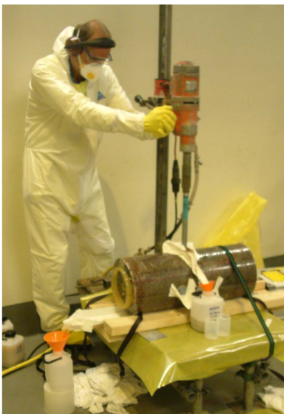
Drilling of sample cores from matrix rock surrounding the test section in the small diameter extension borehole.
