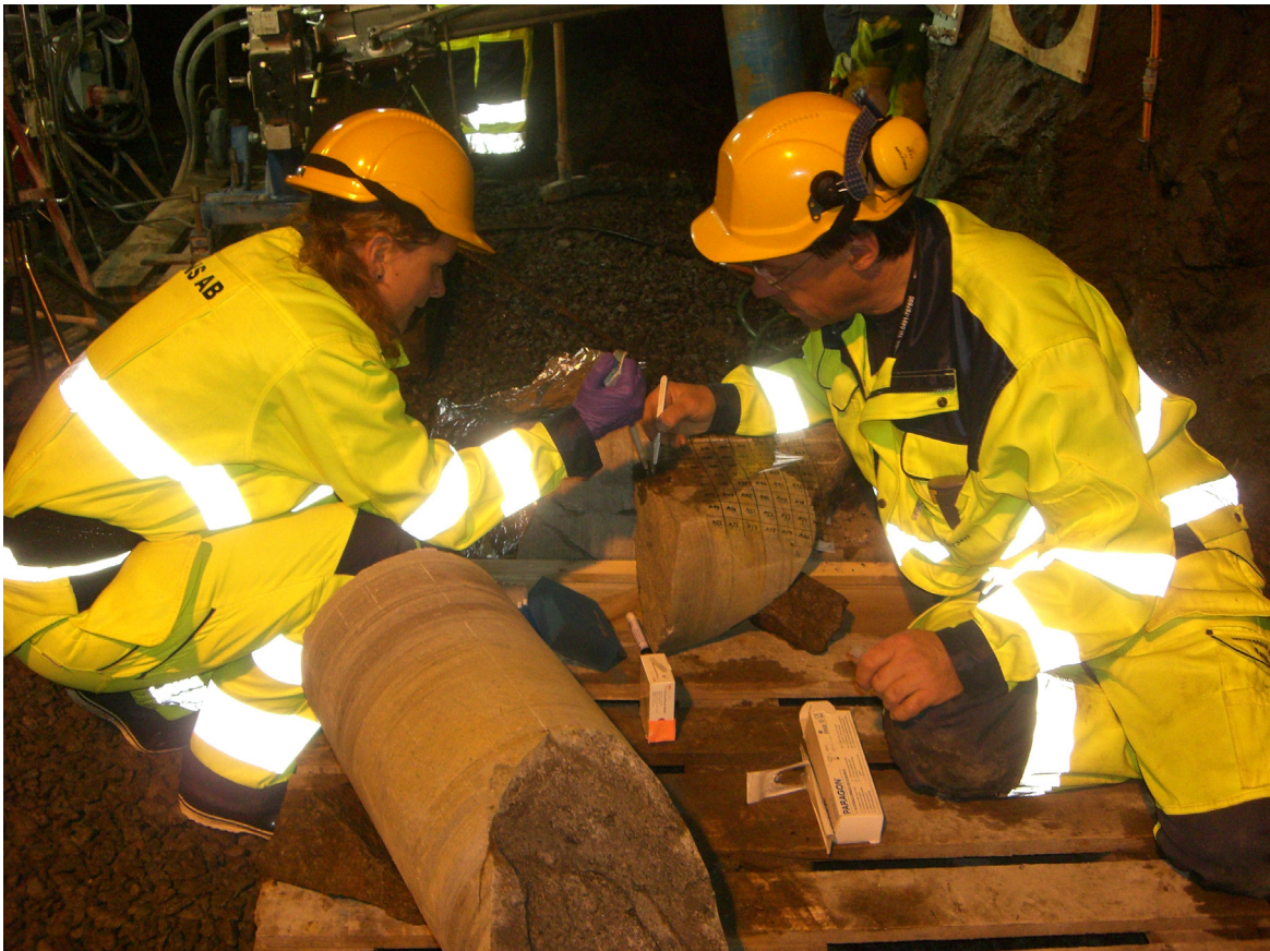
Figure 3-1. Sampling of a fracture surface for analysis of DNA and RNA in biofilms. Tracer Retention Understanding Experiments.
